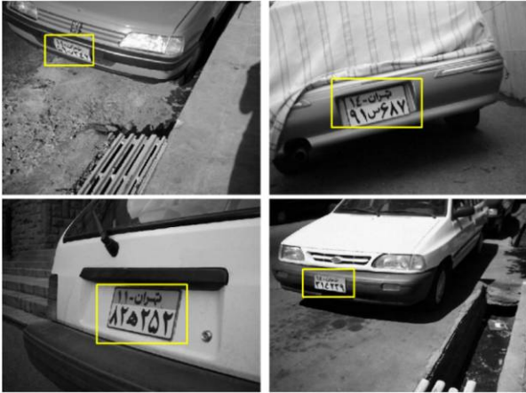
Fig. 5. Results of the proposed algorithm for four lasery license plates with different imaging geometry.
